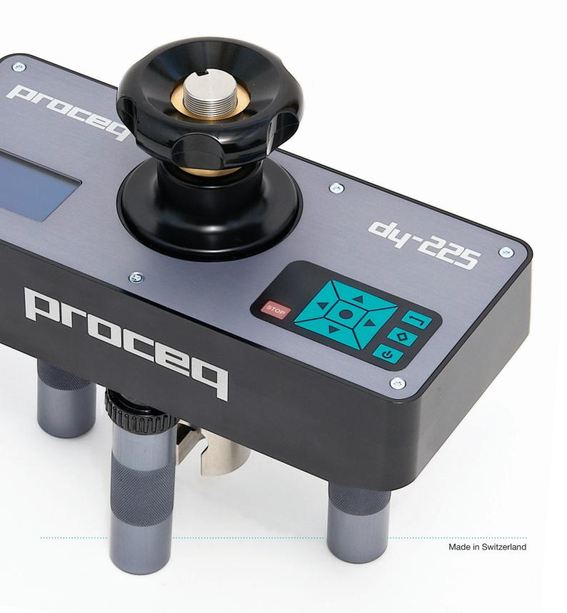
The Proceq DY-2 family of automated pull-off testers covers the complete range of pull-off applications with unmatched ease of operation and a unique capability to store a complete record of the test.
